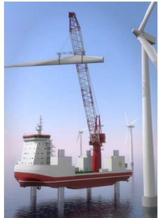
Wind turbine service jack-up vessel. Illustration courtesy OSK-Ship Tech.
