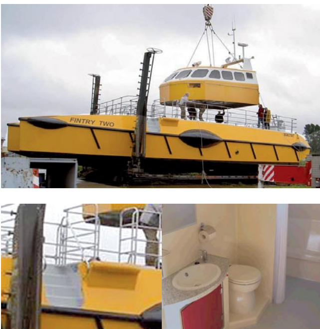
FIGURE 8 Sandwich panels are suited not only for the hull construction, but are recommended in particular to make single modules, whole cabins, superstructures, deck furniture and even stairs separately and to integrate into the construction (on the left: Module construction of the hulls and the cabin of the P200 of pilot's catamaran; middle: Stairway steps and deck projection; on the right: Inside elements from GRP-sandwich panels in a houseboat).
