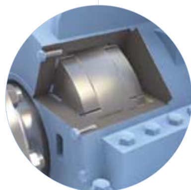
The thrust bearing is of the tilting pad type, absorbing the propeller thrust in both ahead and astern direction.
