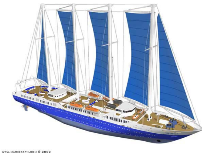
Fig 2: Example for an INDOSAIL rig Ex Cruise vessel project INDIGA, 2005 Geesthacht
